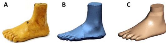
Figure 1. Jaipur foot modeling; (A) real foot; (B) scanned foot-STL file; (C) final model-CAD file Source: Created by the authors
