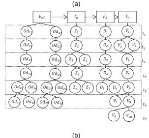
Figure 5. Task graph for MIMO-OFDM architecture, (a) transmitter, (b) receiver
