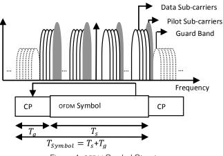
Figure 4. OFDM Symbol Structure.
