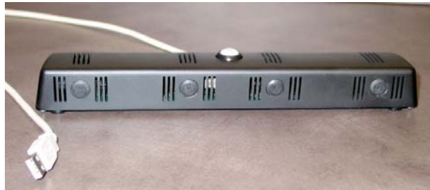
Figure 9. Linear four-element USB microphone array.
