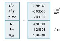
After a deflection and deformation in the structure, proceed to determine the safety factor, knowing the thickness of each layer of the material is 0.325 mm. These values were determined to be 5 layers were used which increase the thickness of 1.625 mm sandwich safety factors.
