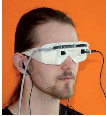
Figure 2. Subject wearing the device PERSEUS with stereoscopic cameras and integrated headphones. Heavy limitation of this device is only 6.5 meters long wired connection between the operator and the subject.
