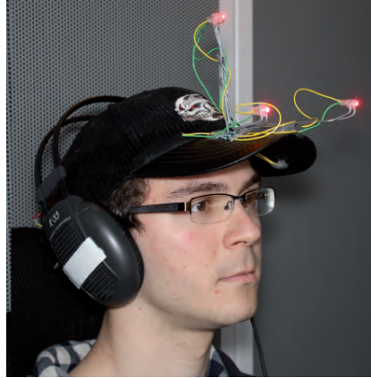
Figure 8. Subject during performing dynamic localization test. Head Tracking for system for head motion compensation consists of cap with LED triangle and computer with web camera.
