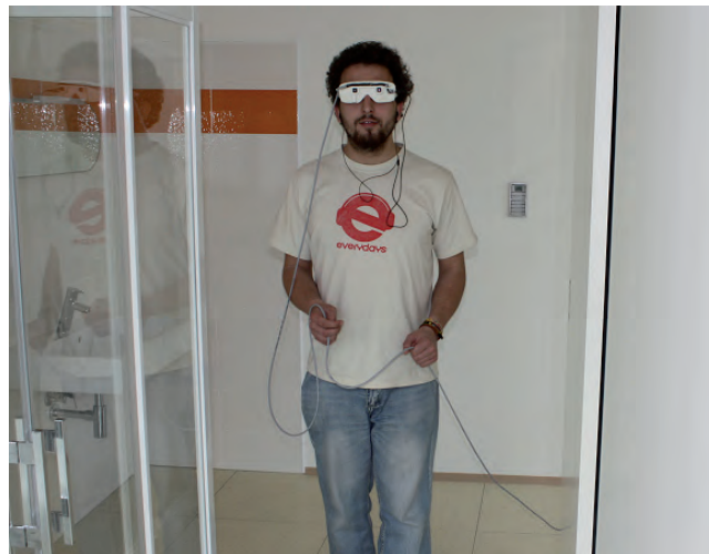
Figure 5. Blindfolded subject wearing navigation system nearly reaching the destination. Wired-base limitation of the system prototype is obvious.
