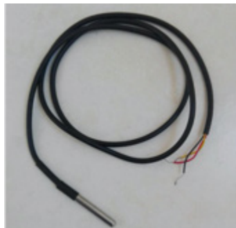
Figure 5. Temperature sensor DS18B20
