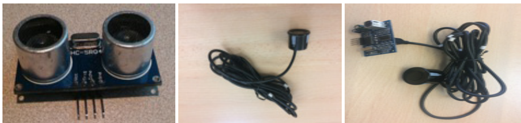
Figure 1. (Top left) HC-SR04 sensor, (top-right) ultrasonic transducer, (down) JSN-B02 sensor.
