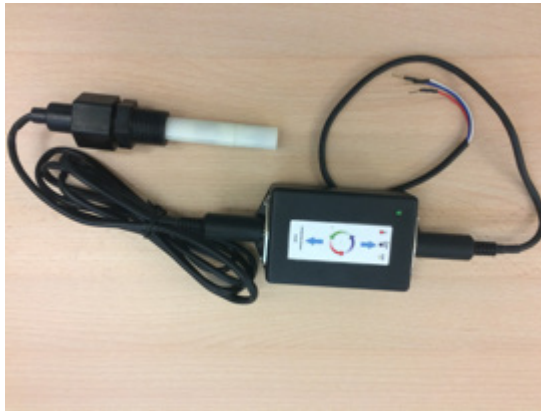
Figure 4. Salinity sensor A1002v1
